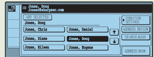
With LDAP, users only need to enter the first few characters of the destination e-mail address—so sending a file is incredibly quick.
